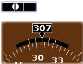
True gyro and accelerometer based slip and turn rate. Plus GPS ground track
