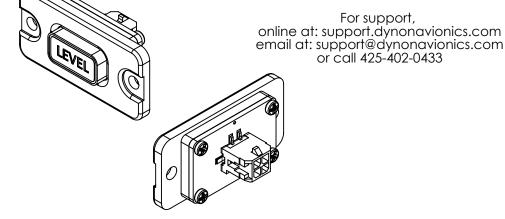
SkyView SV-LEVEL-BUTTON Panel Cut-Out and **Connection Detail**
